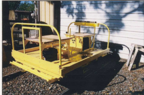
There is another railroad motor car undergoing restoration and assembly at the Railroad Park. This is our Fairmont Model S-2 car. Rick Aubin has begun assembling the car using only photos for a guide. Hopefully we'll find a schematic and/or Rick will be able to figure it all out. This photo was shot from inside our SP Section Tool House.—Tony Johnson photo
