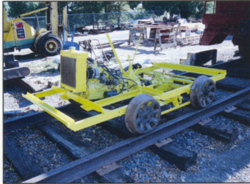
In this September 24 photo the seats, fuel tank, engine cover, operator's seat, end bars and more are in place, Ken Hill did a wonderful job of installing all new wood on the deck and seats. It looks great! - Tony Johnson photo
