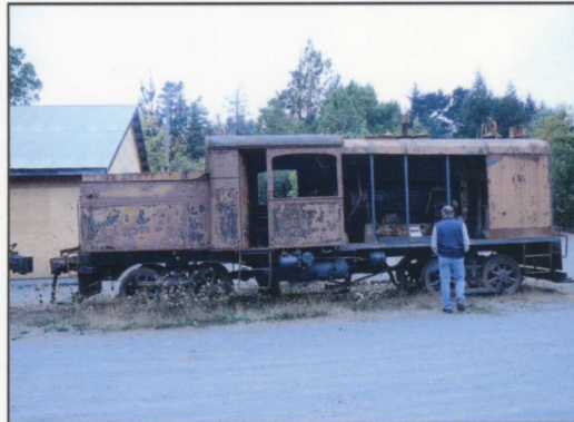
Probably the most unusual locomotive at the Glendale storage yard is Mutual Plywood Corp No. 54, converted to diesel from a 24-ton 2-truck Heisler. Originally built as Elk River Mill & Lumber Co. No. 3, it worked for only 10 years until the mill shut down for good. A junk dealer scrapped the boiler and sold the rest to Mutual Plywood Corp., where they mounted a Murphy diesel engine on the frame and used it as a mill switcher. In the 1960s it became U.S. Plywood Corp. No. M62.—Art Turner photo
