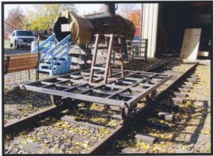
Sitting outside our locomotive shelter is the nearly completed frame and running gear on our homemade handcar. Not long after the photos was taken the handlebars and safety railing were mounted. A wooden floor will cover the deck after the metal is cleaned and painted.
