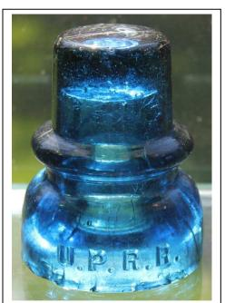
Jumping forward to the late 1860's, the insulator technology had advanced to a threadless pin type glass insulators. On the transcontinental railroad being built by the Union Pacific through Wyoming and Utah the railroad used an insulator manufactured by Mulford & Biddle embossed U.P.R.R. and appeared in
