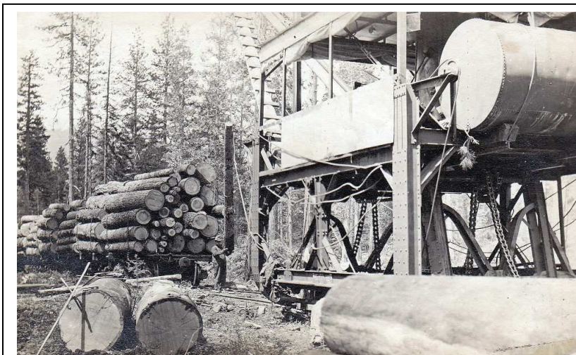
Two recently donated photos from the Gold Hill Historical Society from descendants of the railroad owners show a McGiffert log loader at work. The donors think they show the operation on Sardine Creek, but that was a two-foot, narrow gauge operation. I believe this is actually the company's standard gauge operation on Kanes Creek.
